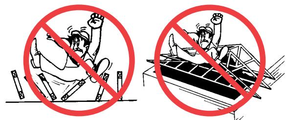
**DANGER** Do not walk on unbraced trusses.
